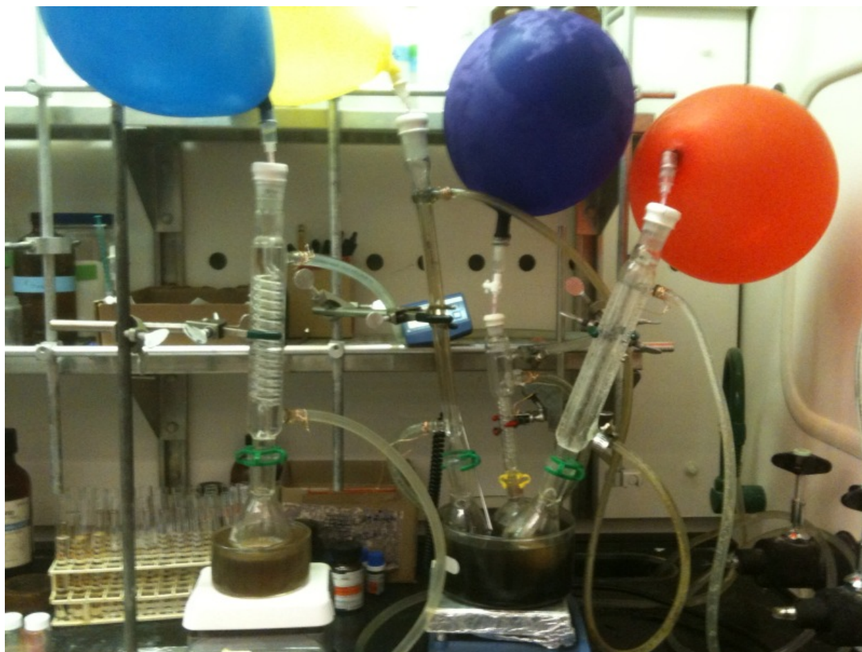
Figure 3. More examples of using nitrogen-filled balloons to protect the reactions from atmosphere.
